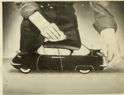
Rub down last lacquer coat with rubbing compound and polish with hard wax.
